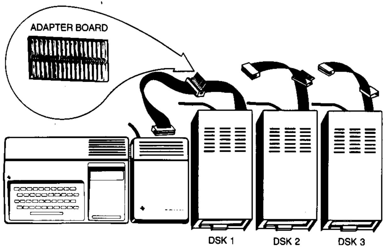
The first drive, the one connected directly to the controller, is identified as DSK1 by TI·BASIC. The second drive, connected to the cable of DSK1, is DSK2. The third drive is DSK3. The labels provided with your drive(s) can be used to identify each drive.
