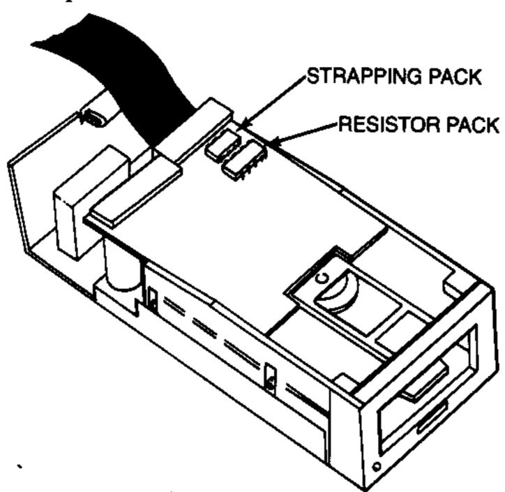
4. Remove the termination resistor pack by prying each end up slightly with a small screwdriver and then lifting it out by your thumb and forefinger. Pull straight up.
